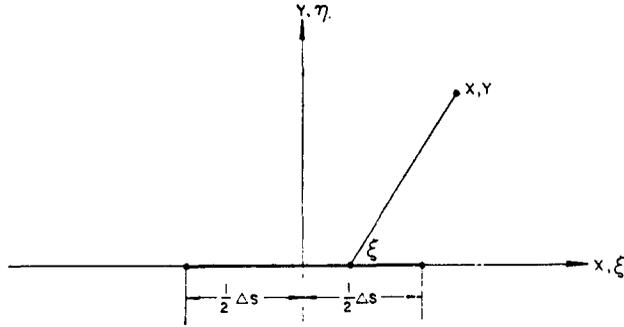
FIG. 5. Integration over a line-segment element for the two-dimensional case.
