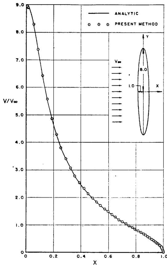
FIG. 21. Comparison of analytic and calculated velocity distributions on an elliptic cylinder of thickness ratio 8.
