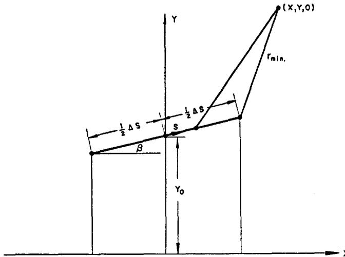
FIG. 7. Integration over a line-segment element for the case of an axisymmetric body.
