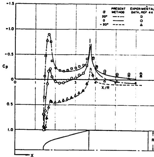
FIG. 46. Comparison of calculated and experimental pressure distributions on a blunted  $15^\circ$  cone-cylinder at  $0^\circ$  and  $\pm 20^\circ$  angle of attack.
