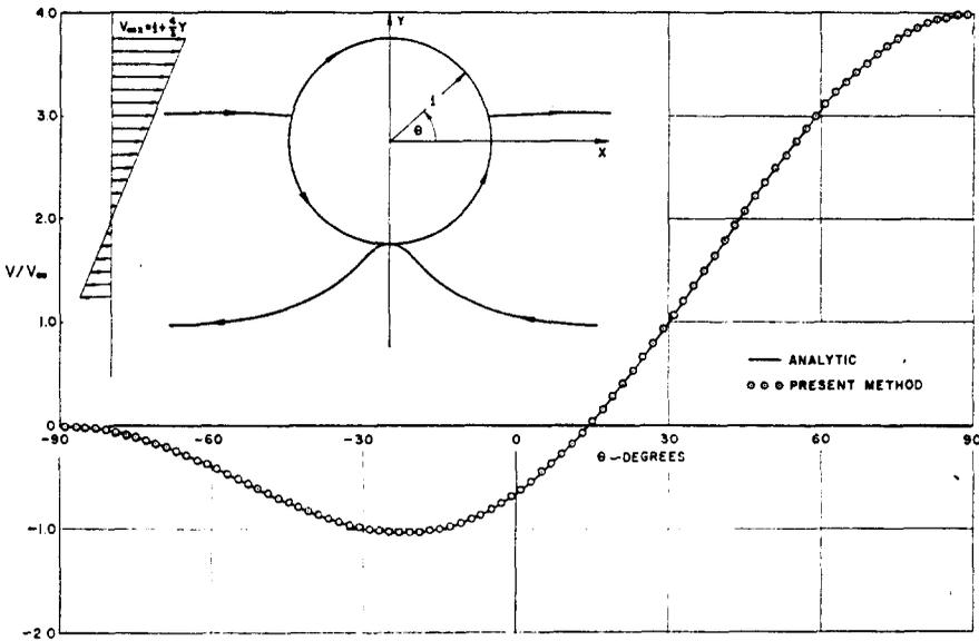
FIG. 26. Comparison of analytic and calculated velocity distributions on a circular cylinder in a uniform shear onset flow.
