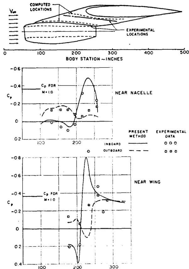
FIG. 57. Comparison of calculated and experimental pressure distributions on a DC-8 pylon in the presence of the nacelle and wing at a free-stream Mach number of 0.825 for the zero-lift condition.
