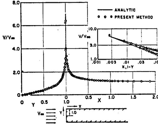
FIG. 22. Comparison of analytic and calculated velocity distributions on a semi-infinite two-dimensional body of rectangular cross-section. Insert shows log-log plot of velocities near corner.
