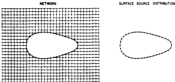
FIG. 19. Control points for network and surface source distribution methods.
