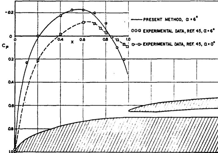
FIG. 48. Comparison of calculated and experimental pressure distributions on an NACA 1-60-060 spinner in an NACA 1-70-100 cowling.
