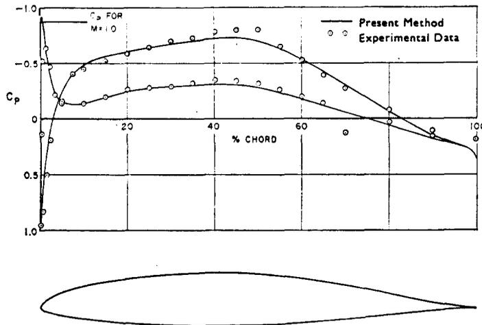
FIG. 38. Comparison of calculated and experimental pressure distributions on an airfoil at a lift coefficient of 0.25 for a free-stream Mach number of 0.68.
