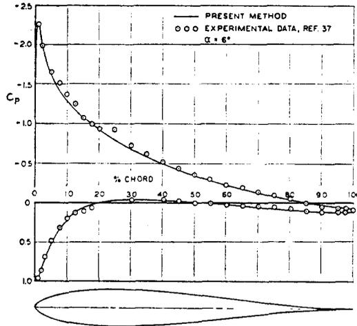
FIG. 37. Comparison of a calculated pressure distribution corrected for boundary layer effects with experimental data for an 11.8 per cent thick Joukowski airfoil at  $6^\circ$  angle of attack.
