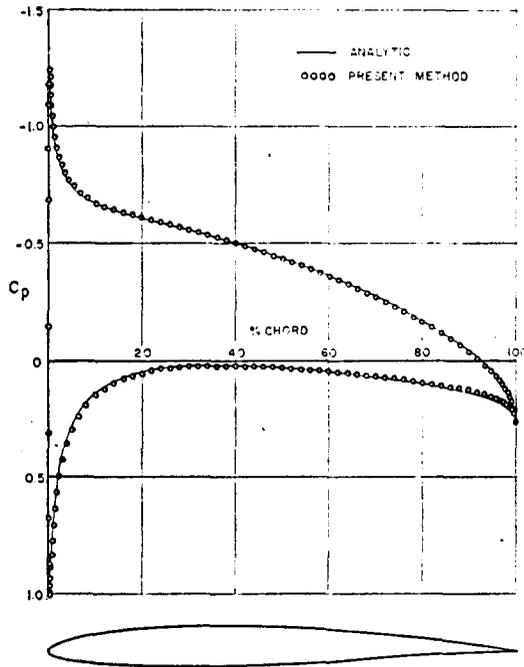
FIG. 24. Comparison of analytic and calculated pressure distributions on a Kármán-Trefftz airfoil at a lift coefficient of 0.5.
