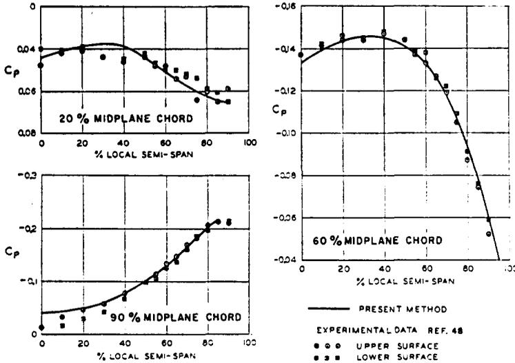
FIG. 54. Comparison of calculated and experimental spanwise pressure distributions on a symmetric delta wing at zero lift.
