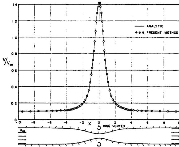
FIG. 30. Comparison of analytic and calculated velocity distributions on the wall of an axisymmetric duct generated by superposition of a ring vortex and a uniform stream.
