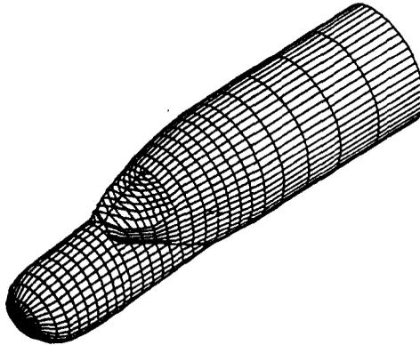
FIG. 50. Elements used to approximate a C-135 fuselage with a large radome. (Unretouched output from an automatic plotter.)
