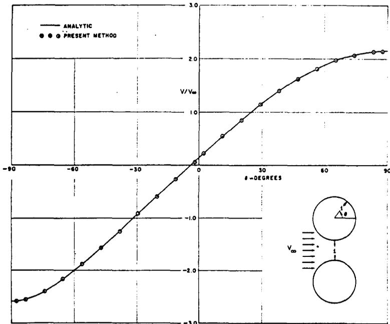
FIG. 25. Comparison of analytic and calculated velocity distributions on one of two identical circular cylinders whose centers are one and one-half diameters apart.
