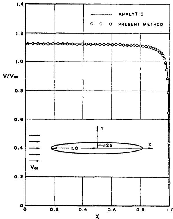
FIG. 20. Comparison of analytic and calculated velocity distributions on an elliptic cylinder of thickness ratio  $1/8$ .
