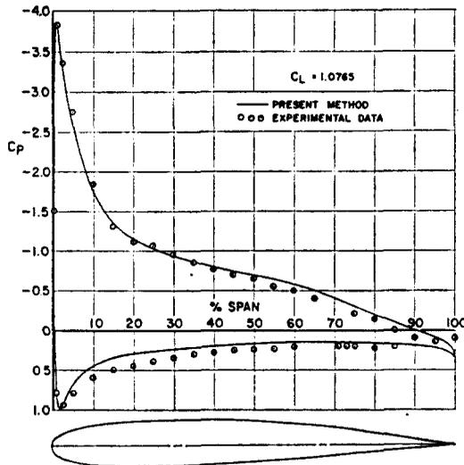
FIG. 35. Comparison of calculated and experimental pressure distributions on a Douglas DSMA 387 airfoil at a lift coefficient of 1.0765.
