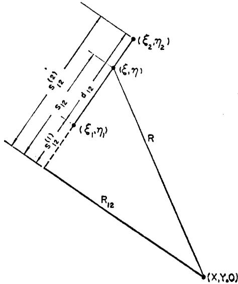
FIG. 12. Integration over a side of a quadrilateral.
