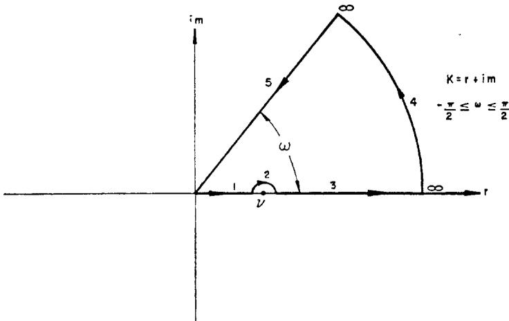
FIG. 16. Contour integration for obtaining a purely real exponential. Line 1, 3, is the original path. Line 5 is the one for which the exponential is purely real.
