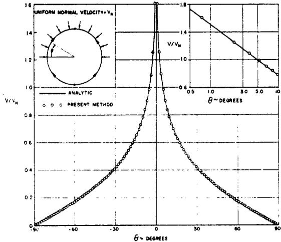
FIG. 23. Comparison of analytic and calculated tangential velocity distributions on a circular cylinder having a discontinuous normal velocity distribution. Insert is a semi-log plot of velocities near the discontinuity of normal velocity.
