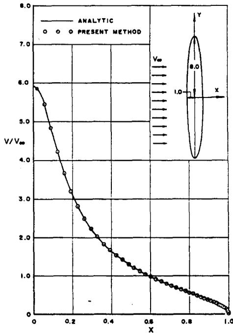
FIG. 28. Comparison of analytic and calculated velocity distributions on an oblate spheroid of thickness ratio 8 in axisymmetric flow.
