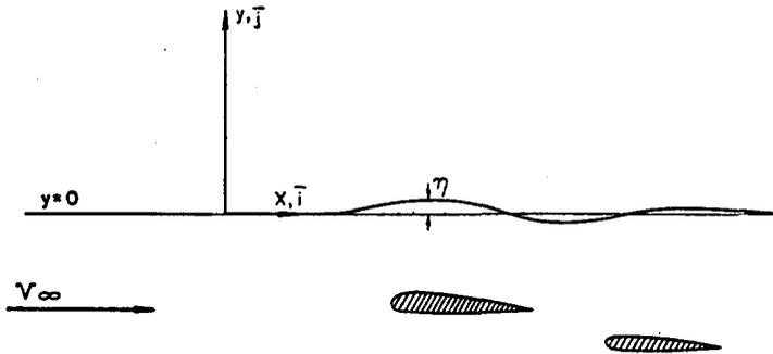
FIG. 13. Diagram for analysis of flow about hydrofoils.
